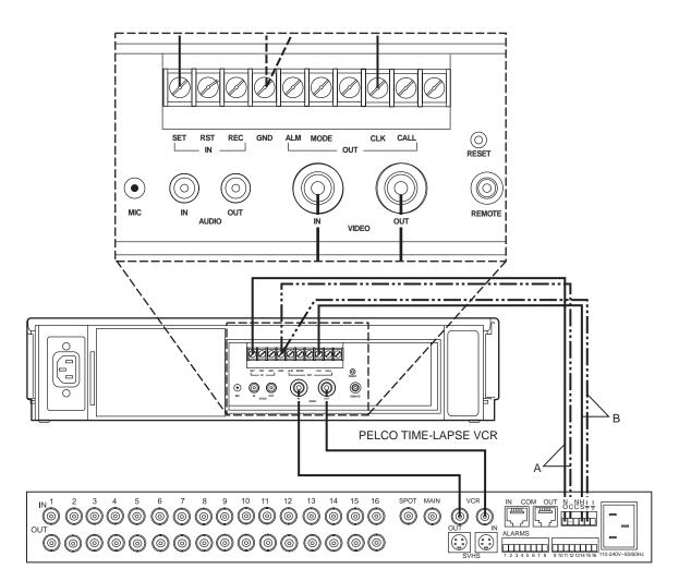
Figure 7. Pelco Time-Lapse VCR Wiring Example
